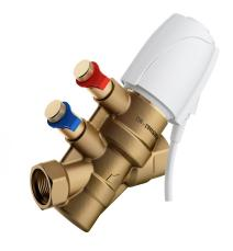
A combination pressure independent flow control valve (PICV) with adjustable flow setter, integrated measuring venturi, and differential pressure regulator. The ND comes standard with two pressure and temperature test plugs, and a universal actuator mounting collar.
