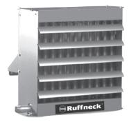
The Advanced Horizontal unit heater exchanger can be customised for your application. The heat exchanger is comprised of extruded finned tubing in 10, 9 and 5 fins per inch for varying steam conditions and/ or where atmospheric particulate may cause premature fouling of the heater core. Additionally, the AH can handle more pressure than the HP and FR.
