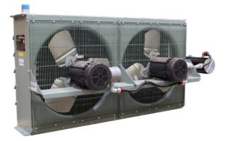
The dual fan arrangement allows for two smaller fans that can be operated at the standard 1725 RPM. Furthermore, dual fans provide for output modulation if separate motor thermostats are used. Separate motor thermostats produce better control of heating during periods of low demand by reducing the output of the heater.
